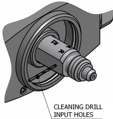
Cleaning "Round" Chamber Product Input Holes
