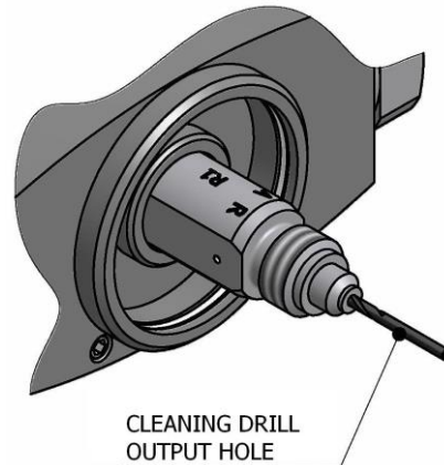
Cleaning "Round" Chamber Product Output Hole
